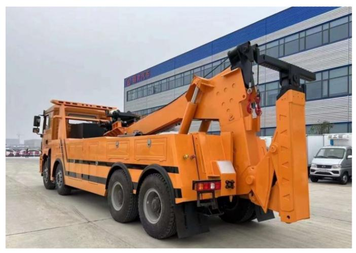
30 tons 360° rotator wrecker body
